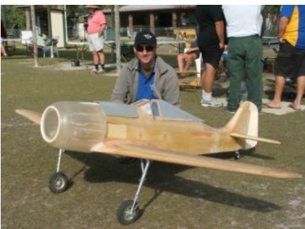
102" Meister Plan FW 190 A8 - A Moki 150 radial is to be fitted. Chris Lawn - Bundaberg 2014
